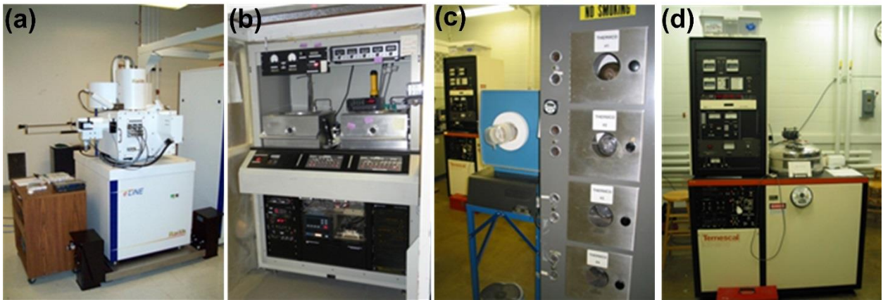
Figure 2.1 Major fabrication equipment used in this research. (a) Raith e-beam lithography system. (b) Reactive ion etching system. (c) Oxidation and ion diffusion furnaces. (d) E-beam evaporator system.
